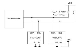
Figure 2. Typical System Configuration
