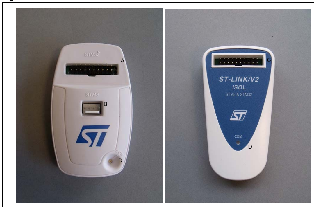
Figure 4. Connectors of the ST-LINK/V2 and ST-LINK/V2-ISOL
