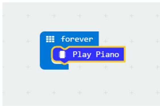
Go to “Basic”, and place “forever” slot into the blank space on the right. Place the “Play Piano” block of WSTouchPiano inside the “forever” slot. Click “Download” button on the bottom left to save the project, move the .hex file to the micro:bit drive to transfer the code into your micro:bit, and insert micro:bit to Piano's interface module. Now, you can observe our experiment outcome!
