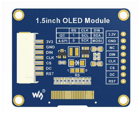
By default, the module is in 4-wire SPI communication mode, that is the BS is connected to 0. Not all the 0 and 1 stands for level, it just stands for the connecting options of the resister. The actual hardware connection for different communication mode is as below:
