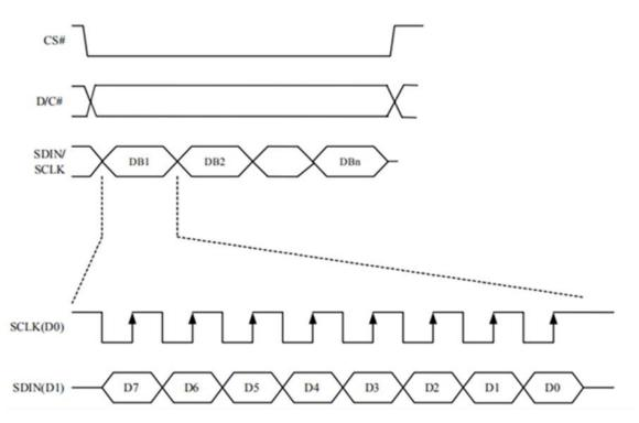
**Note:** The difference between the traditional is that: the OLED only supports display, so we only require the data input (MCU to module) and hide the data line that sends data from slave device to master (MISO). The table can be get at Datasheet Page 21.
