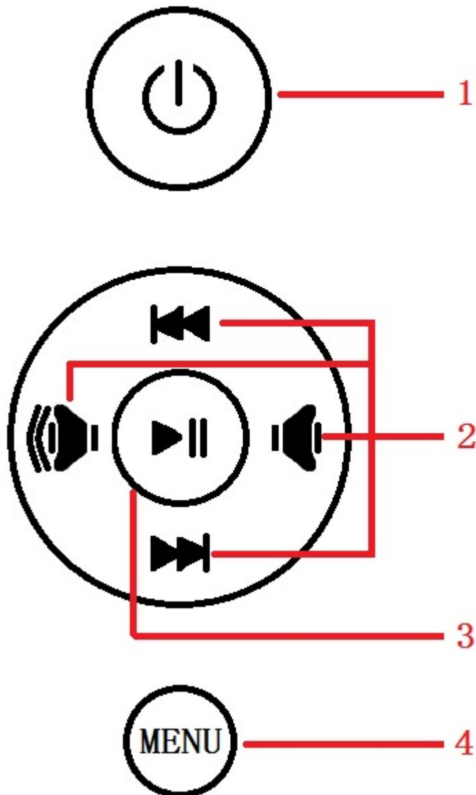
1. Open or Close LCD display. If you don't need the LCD for long time, you can use this button to reduce consumption
