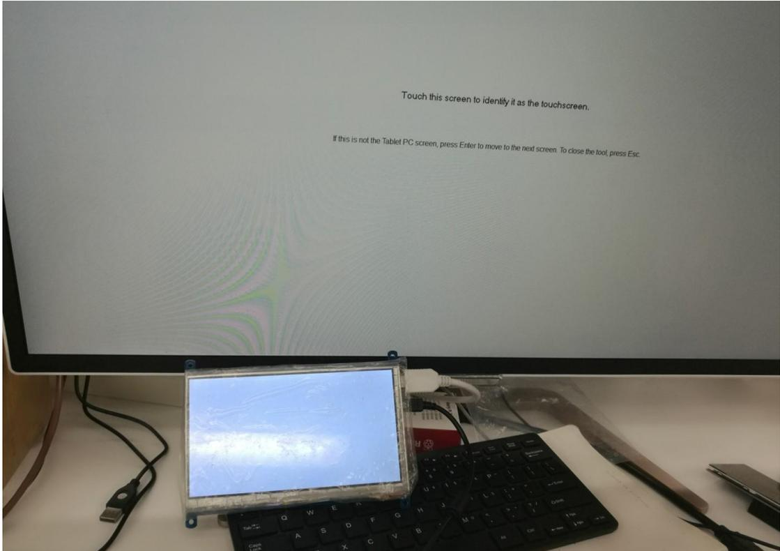
5. Press "Enter" on keyboard, this operation work as tell the PC this screen is not the touchscreen I want to control. Then, you can find that the prompt has turn to
