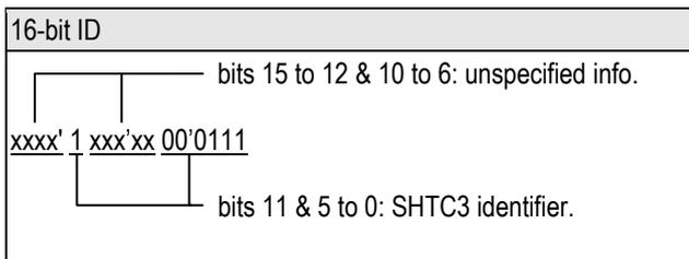
**Table 15** Structure of the 16-bit ID. Bits 15:12 & 10:6 of the ID contain unspecified information (marked as “x”), which may vary from sensor to sensor, while bits 11 & 5:0 contain the SHTC3-specific product code.
