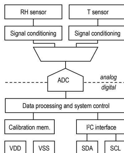
Figure 1 Functional block diagram of the SHTC3.
