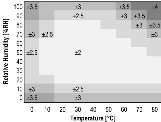
**Figure 4** Typical accuracy of relative humidity measurements given in %RH for temperatures 0°C ... 80°C.
