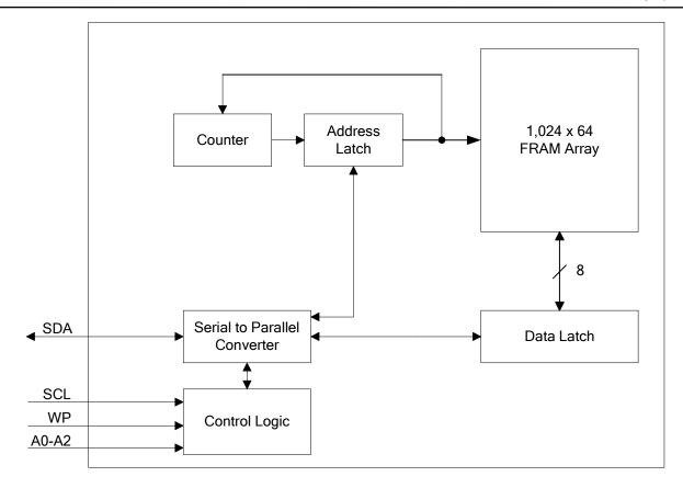
Figure 1. FM24CL64B Block Diagram
