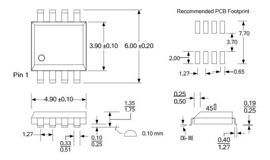
Refer to JEDEC MS-012 for complete dimensions and notes. All dimensions in millimeters.
