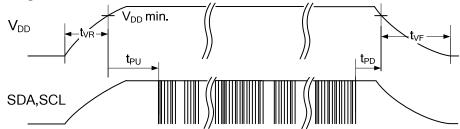
**Power Cycle Timing** ( $T_A = -40^{\circ}\text{C}$  to  $+85^{\circ}\text{C}$ ,  $V_{DD} = 2.7\text{V}$  to 3.65V unless otherwise specified)
