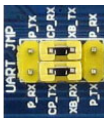
Figure 7: Jumpers setting for serial debugging function between the Pi and the XBee
