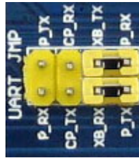
Figure 14: Setting jumpers on ARPI600
