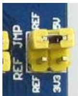
Figure 18: Setting AD reference voltage
