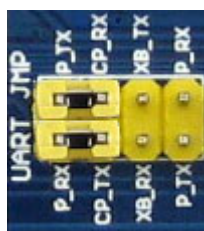
Figure 2: Starting up serial debugging function
